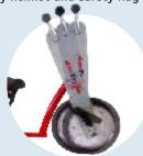
Hinged front end with three positions for adjustable hand crank/foot crank to seat alignment.
